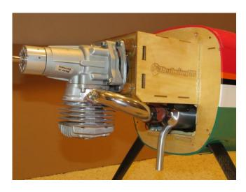
Engine, header and canister installed. Note coupler between header and canister. Also note a small corner of the motorbox was cut off to clear the header. This was cosmetic only and did not affect strength at all.
