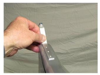
Main gear is installed using nuts and bolts that are inserted in predrilled holes. Bolts go through landing gear cover, main gear, then fuselage bottom. Nuts are installed inside the fuselage and accessible via the canister tunnel. Note: remove covering from landing gear cover at four bolt positions.
