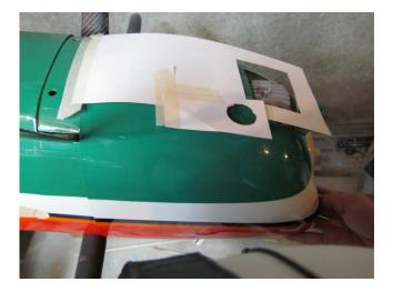
Reinstall cowl. Transfer position of the muffler stack to the cowl. Note: the cutout for the engine head goes just past the spark plug.
