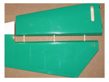
Inject adhesive into all holes and onto the barbs of all hinges. Make sure all hinges will go in holes. Push elevator into position. Once hinges are properly seated, rock elevator back and forth a few times to help align hinges.
