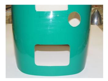
Cut the opening for the muffler stack. While you are at it, cut the exhaust opening.
