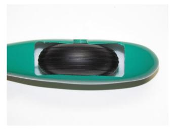
Install axles on main landing gear. Note: the wheel pants have a tight fit on the axles. The axles need to be oriented so flat sides are vertical (points are up and down). Wheel pants have a very tight fit with wheels. The wheel pants have to be opened up to fit the wheels properly.
