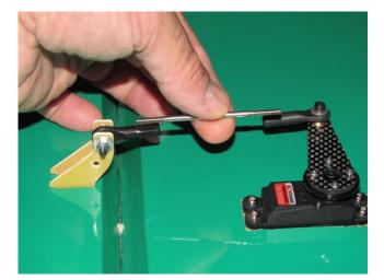
Prepare servo arms. Carbon fiber arms are provided for all control surface servos. The round wheels that come with the servos can be used. If desired, aluminum wheels can be purchased from RedWing RC for an additional cost. These wheels are drilled and tapped to fit the arms.
