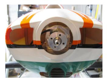
Check to see how the engine fits the cowl. There must be a difference in centerline between the DLE and DLA engines. Cowl will not line up properly with spinner backplate.
