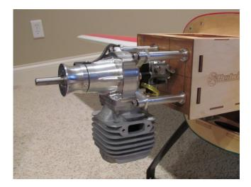
Install standoffs but don't use thread lock on bolts yet. Note: a 10 mm open end wrench fits on the flats of the standoffs. Temporarily mount engine.
