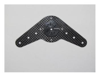
Mounting holes in the carbon fiber arm do not line up with the aluminum wheel and must be drilled. Use a small drill bit and drill through the desired holes in the wheel. Once all holes are drilled, remove the aluminum wheel and redrill the holes in the CF arm with the proper size. Bolt aluminum wheel to CF servo arm.
