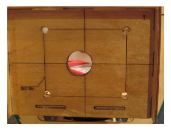
A DLA-58 is being installed on this Slick. The bolt pattern is slightly different than the DLE-55. Mounting holes were adjusted and drilled accordingly.
