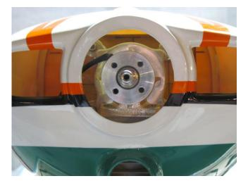
Mounting holes were revised to center the engine within the cowl opening. It looks OK now. Remove cowl. While engine is still mounted, remove standoff bolts (from firewall) one at a time and add threadlock. Reinstall all four standoff bolts.
