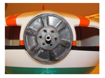
Carefully remove spinner backplate and cowl. Draw circles around the standoffs. Mounting holes will be drilled in the center of the circles. In this case, holes were drilled through the dowels and firewall. Spinner backplate should line up like this.
