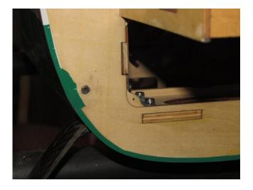
Reinstall cowl. Upper bolts are accessed from the canopy side. Bottom bolts are accessed from inside cowl and are difficult to install. Exhaust opening can be used to access bolts. Bottom nuts and bolts can be replaced with rare earth magnets. Use one magnet on cowl ring, one on the fuselage. Remember to arrange magnets to attract, not repel. We also put a bolt at the bottom center of the cowl ring.
