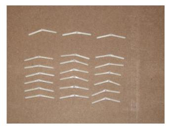
Remove all hinges from their pre-drilled holes. Scuff barbs on all hinges with coarse sandpaper or similar tool. Note: two hinges have had one barb clipped off. The short side of these two hinges go into the stabilizer in the hole closest to the fuselage.
