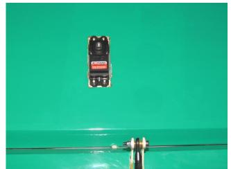
Reinstall aileron servos. Use 18" (or 12" with 6" at receiver) extension on servo lead. Don't forget to use some sort of restraint on the connector. Restraints are commercially available. Dental floss can be wrapped around the connector and tied 3 or 4 times. Some people like heat shrink tubing. If heat shrink is used, avoid overheating the connector. Install aileron servo. Note: servo spline is closer to the leading edge of the wing.
