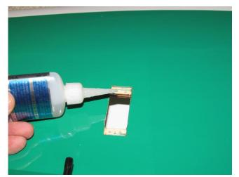
Verify control horns have cured prior to installing servos.
