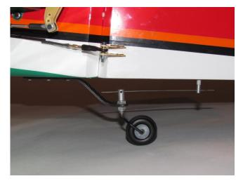
Only one wheel collar is given in the kit for the tail wheel. A washer was soldered onto the axle to center the wheel. A second washer was soldered as a stop to keep the axle from riding up the tail wheel bracket too far. File a flat spot for the wheel collar.
