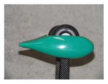
Wheels and wheel pants installed. Note: when properly aligned, the front pant hides the back one.
