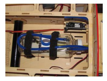
Tank is strapped in with Velcro. Vent line loops back over the end of the tank prior to exiting out the motorbox bottom.
