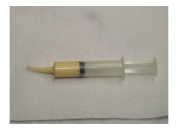
Several different types of adhesive are acceptable for installing hinges. Epoxy, Gorilla Glue and aliphatic resin (Titebond II) all work. One benefit of the aliphatic resin is it cleans up with water until it cures. A dental syringe is an excellent tool for injecting glue into the holes.
