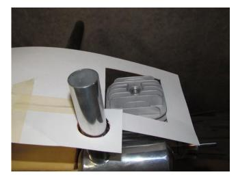
Put head template back on. Add a section to template for the muffler. Carefully remove muffler.
