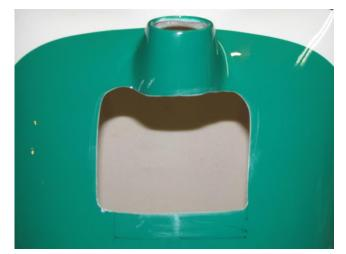
Remove engine and install cowl. Fold template back onto the cowl. Trace outline of engine head onto cowl using Sharpie or similar marker. Fold template back and remove cowl. Make initial cut somewhat smaller than the template shows. The cowl has a pretty steep slope at the engine head location. This opening doesn't have to be as long as the engine head. Trial fit the cowl over the engine. There should be about 1/8" clearance along both sides and the front of the engine head.
