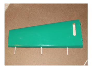
Install all hinges in the flying surface. Make sure all hinges line up the same. If you would like, proceed directly to installing the hinges in the control surface at this time.
