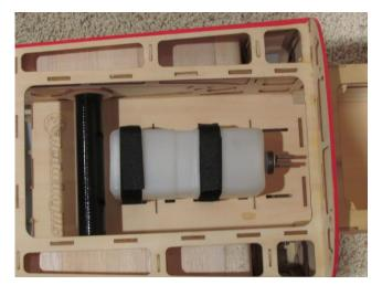
A 550 cc 3 line tank comes preassembled and installed. We opted to use a 16 ounce tank from Fortitude.
