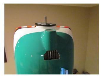
Support fuselage vertically on ladder (or similar). You want the firewall to be horizontal. Place engine on firewall. This is a 3W-55i with a metal mounting plate. These standoffs are short oak dowels. The mounting bolts with go through the mounting plate, dowel and firewall. Set cowl and spinner backplate in position. Cut cowl as required to clear the head fins. Move the engine until the spinner backplate lines up properly with the cowl. Make sure cylinder remains vertical.
