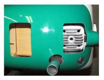
Reinstall muffler using the gasket and threadlock. Install cowl. It may be necessary to enlarge the muffler stack opening for additional clearance to install cowl. There may also be an interference with the front of the muffler like there is in the case of the DLA-58.
