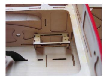
Predrill servo mounting holes in throttle servo mount. Add a drop of thin CA to each hole. Glue servo mount into place.
