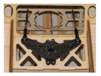
Remove ball link from servo arm. Thread cable end onto ball link. Reattach ball link to servo arm. Install second cable, making sure to cross the cables. Note: getting cables tight enough and centering rudder is a trial and error process. Cables need to be snug, but not "guitar string" tight.
