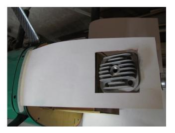
Make a template of the engine head using poster board (or something similar). Tape to fuselage near landing gear. The tape will act as a hinge.
