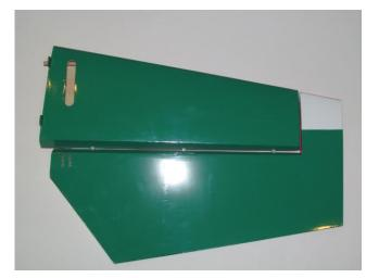
Openings in fuselage for horizontal stabilizer mounting, elevator servo lead and rudder pull-pull cable exit. Slot opened in horizontal stabilizer for the elevator servo arm and elevator slots for control horns.
