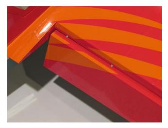
Once all hinges have been installed, clean off excess adhesive. Note: minimal hinge gap and bevel to bevel throw. If necessary, increase hinge gap slightly to achieve desired control throw. Repeat process for aileron and rudder hinges. Note: minimal hinge gap and bevel to bevel throw.
