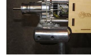
Mark location of throttle pushrod and fuel line. Remove engine (leave standoffs in place) and drill both holes. Reinstall engine. Temporarily mount muffler. In the case of a DLA-58 the muffler interferes slightly with the side of the motor box. A notch had to be cut off. The firewall is completely behind this notch, so the cut is cosmetic only and won't affect strength.
