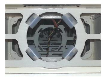
Rear of canister muffler needs to be shock mounted. Install four pieces of silicone in pre-cut mounts. Note – silicone is not included in kit.
